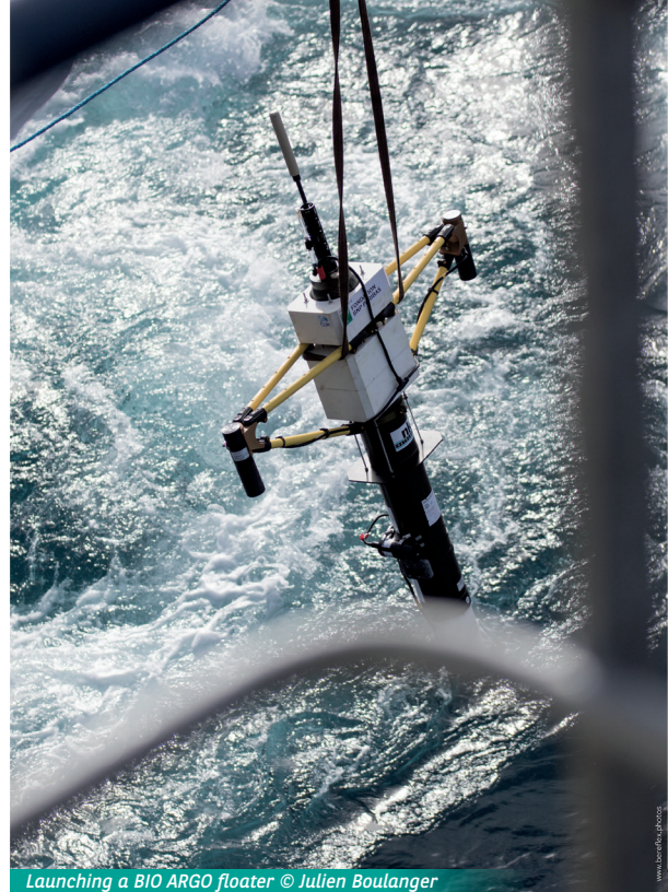
Launching a BIO-ARGO float © Julien Boulanger
