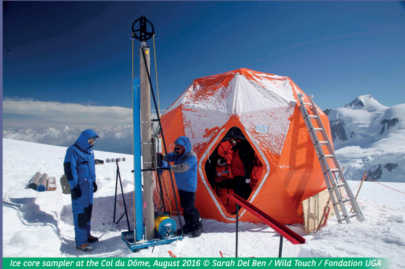
Ice core sampler at the Col du Dôme, August 2016 © Sarah Del Ben / Wild Touch / Fondation UGA
